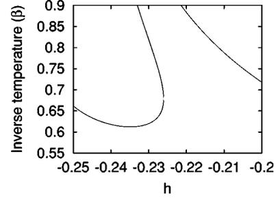
FIG. 3. Numerical solutions of the two-dimensional Migdal-Kadanoff equations for a single layer of the three-dimensional molecular model. The critical temperature  $\beta$  is reported as a function of the field strength  $h$ . The stationary point is at  $h = h_0 = -0.2349$  where  $\beta = \beta_c = 0.6122$ . For  $h > -0.226$  there is no physical solution.
